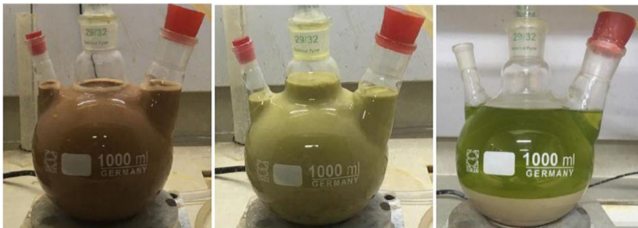
Figure 13. Changes to slurry colour before and after leaching (left to right: before leaching, after leaching and separated solid-liquid, respectively).
