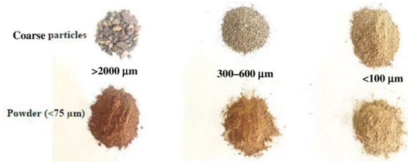
Figure 5. Images of coarse particles and powders of >2000, 300–600 and <100 µm size fractions.
