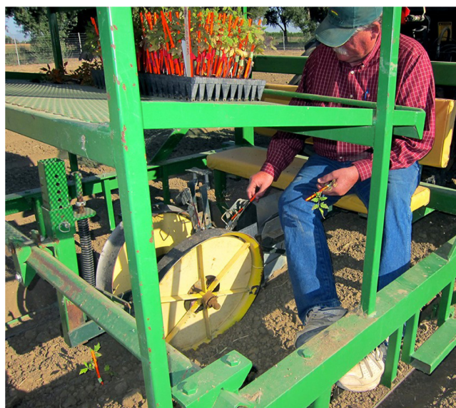
Figure 2. Holland transplanter with butterfly transfer fingers used for transplanting plant labels and tomatoes together.
