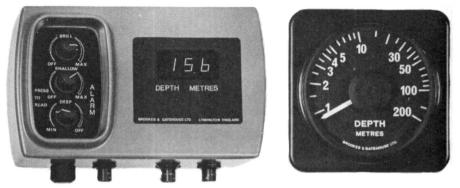
This high powered long range echo sounder with adjustable dual-alarm system gives a digital display of depth. An analogue repeater is available. It has a typical maximum range of 300 metres. In shallow waters this instrument will record depth changes of 10 cms.
