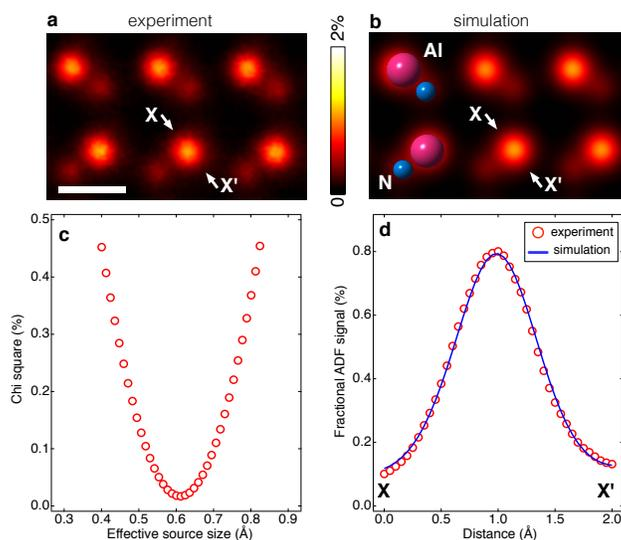
**Figure 2.** (a) Atomic-resolution ADF STEM image of *w*-AlN viewed along *a*-axis (15 atom thickness), where the intensity range is 0 – 2 % of that in the incident electron beam. (b) Simulated ADF STEM image convoluted with a 0.62 Å Gaussian profile. (c) Chi-square test profile as a function of FWHM Gaussian source size. (d) Z-contrast profiles along X-X' for experiment (circles) and simulation (solid line). The scale bar in (a) is 2 Å.
