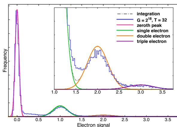
**Figure 1.** The histogram of the corrected background image, where the horizontal axis is the number of electrons. The overlaid profiles are estimated based on Poisson distribution for the discrete events of single, double and triple electrons.
