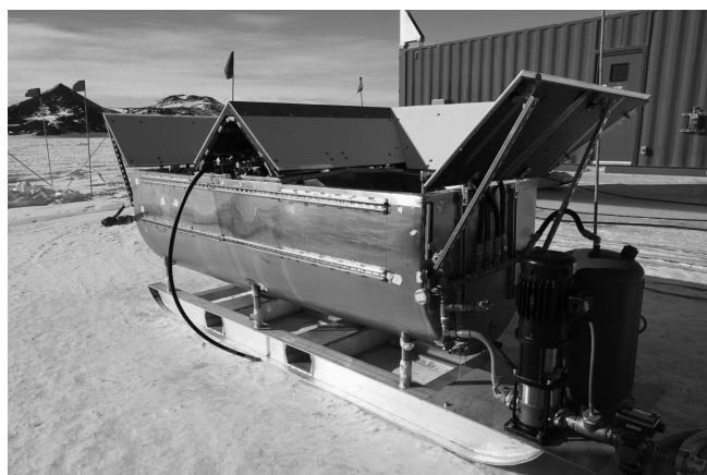
Fig. 2. The finished snowmelt tank showing hopper with exterior bracing. On the right are the pump and expansion tank for the glycol subsystem.
