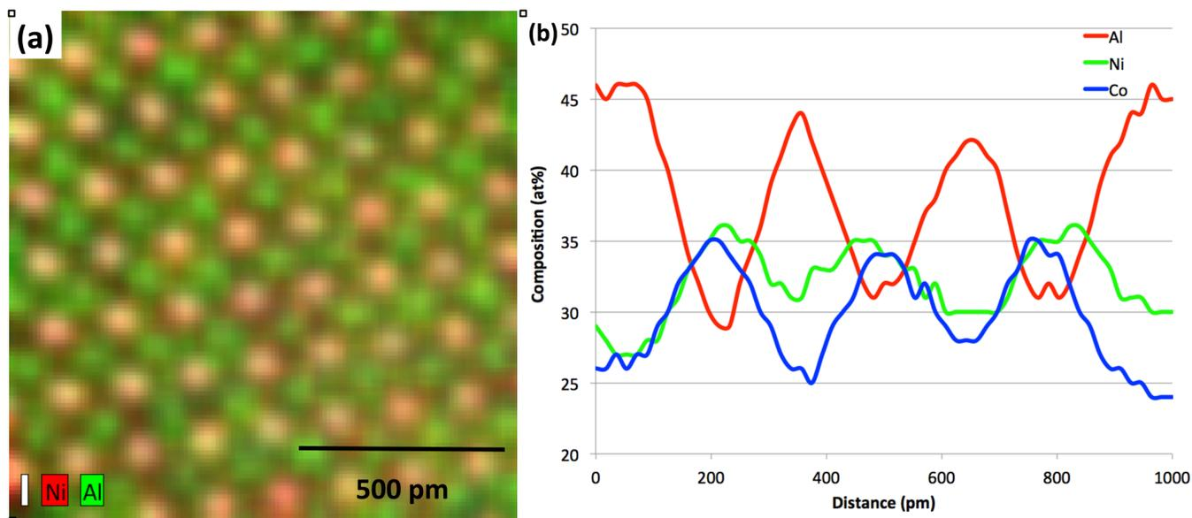
Fig. 1. a) XEDS map (overlaying a HAADF image) of the atomic columns in the model B2 compound with the beam parallel to  $\langle 100 \rangle$ . b) XEDS compositional profiles plotted across a set of columns showing that one of the sublattices consists mainly of Al, while the other mainly Ni and Co.
