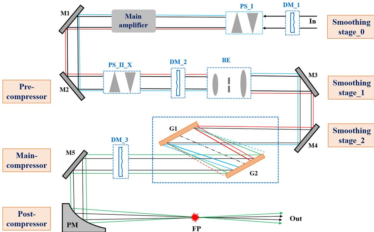
**Figure 4.** Optical diagrammatic sketch of the SSGP-main-compressor-based MPC. PS\_I, PS\_II\_X: prism pair system. DM\_1, DM\_2, DM\_3: reflective deformable mirrors with different sizes. BE: beam expander and relay imaging systems. G1, G2: diffraction gratings. M1–M5: reflective mirrors. PM: parabolic reflective mirror. FP: focal point.
