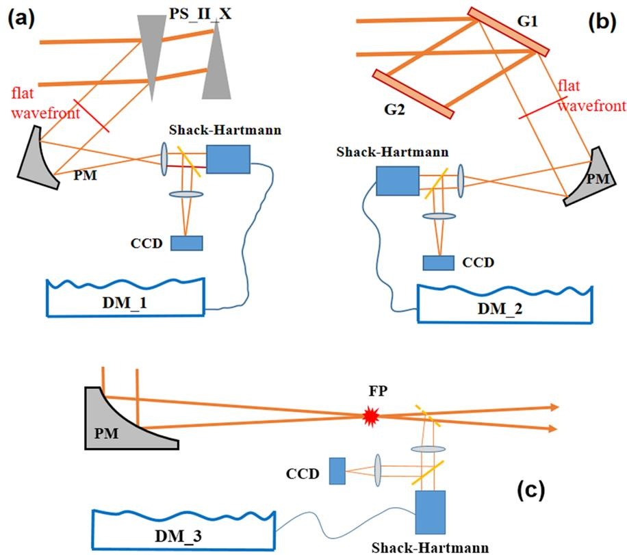
**Figure 5.** Optical diagrammatic sketch for the wavefront aberration measuring and controlling of (a) DM<sub>1</sub>, (b) DM<sub>2</sub> and (c) DM<sub>3</sub>. DM<sub>1</sub>, DM<sub>2</sub>, DM<sub>3</sub>: the reflective deformable mirrors corresponding to Figure 4. PM: parabolic reflective mirror.
