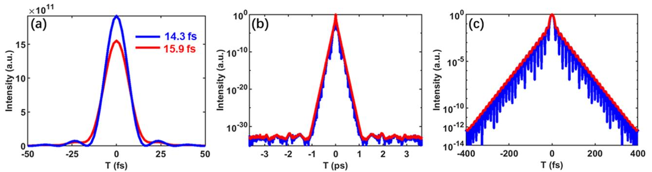
**Figure 8.** (a) Integrated temporal profiles in the focal plane in linear (a) and log (b), (c) scales, where the blue curve represents the ideal condition and the red curve represents the beam output from the SSGP compressor.
