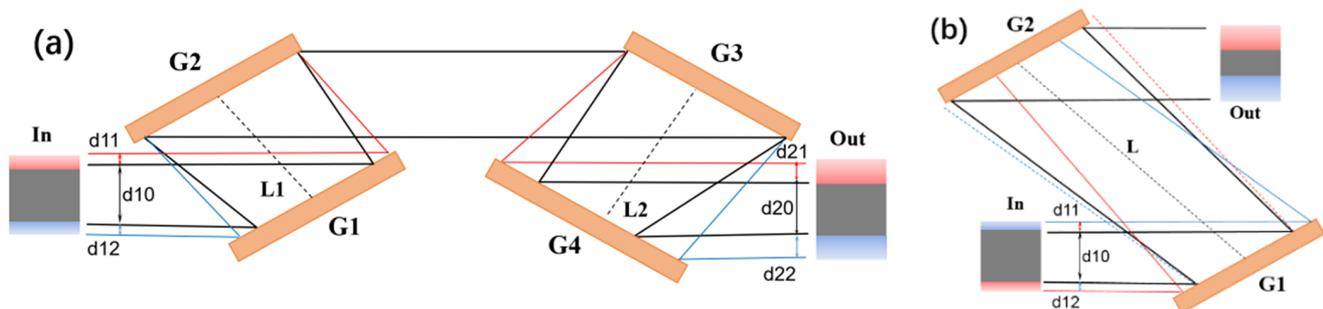
**Figure 1.** Optical schemes of the (a) AFGC and (b) SSGP compressor. G1–G4 are diffraction gratings;  $L = L_1 + L_2$ . In the four beam profiles, the dark gray contain full spectra, and the red and blue areas contain partial longer and shorter spectra, respectively.
