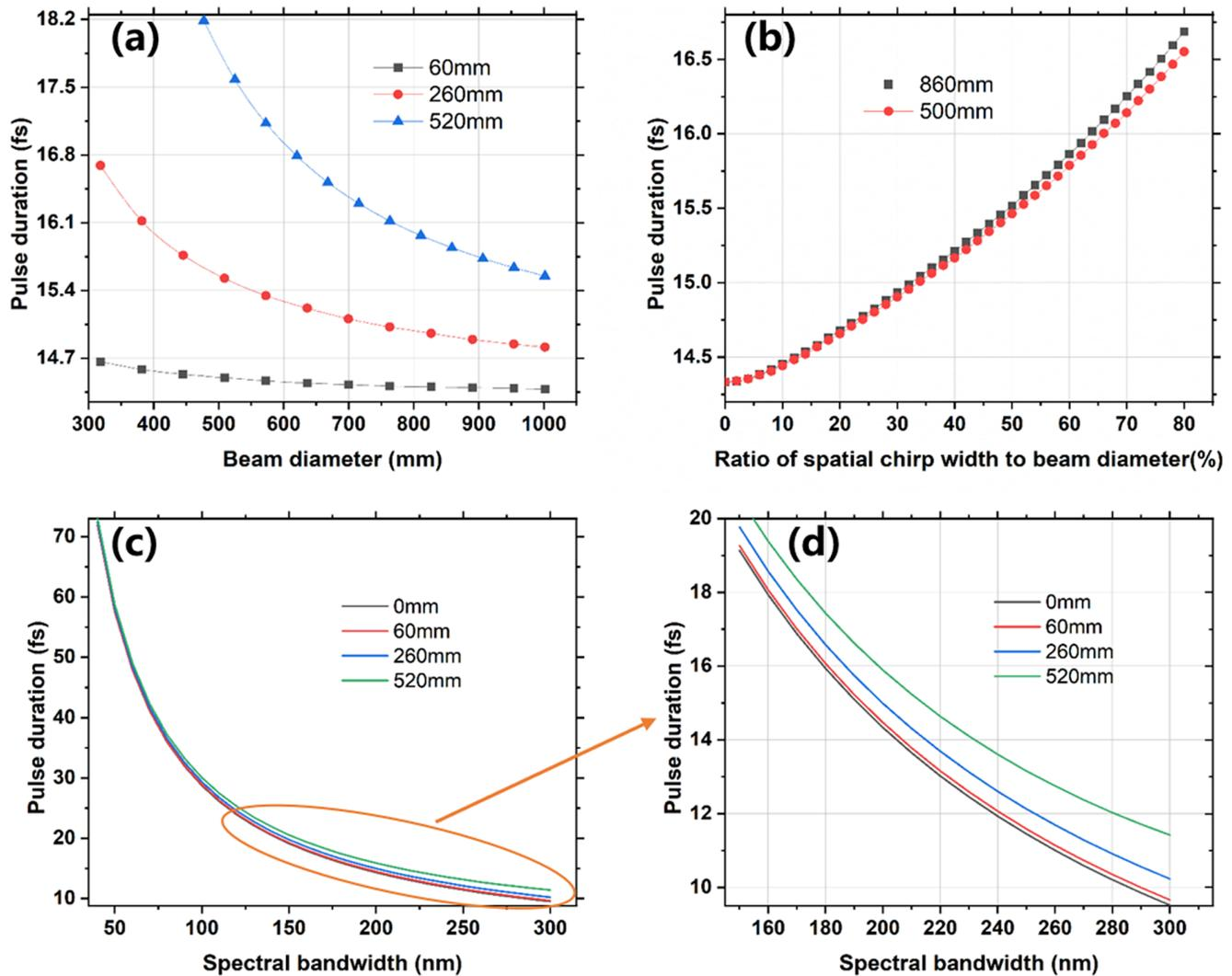
**Figure 9.** Curves of the pulse duration at the focal point related to (a) the beam diameter, (b) the ratio of the spatial chirp region and (c), (d) the spectral bandwidth, at different induced spatial chirp widths (0, 60, 260, 520 mm) and beam sizes (500 and 860 mm), respectively.
