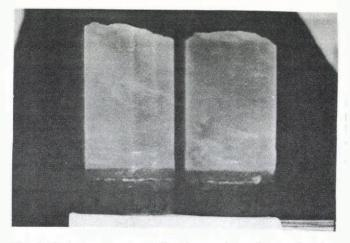
Fig. 3. Laboratory-grown saline ice specimen fractured under tension at -10 °C at  $10^{-7}$  s<sup>-1</sup>. Vertical orientation. Tensile strength: 1.06 MPa. Melt-water salinity:  $3.7^{\circ}/00^{\circ}$  Specimen density: 0.90 Mg/m<sup>3</sup>.
