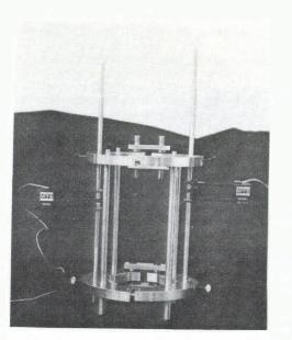
Fig. 2. Extensometer holders which are frozen directly to the ice specimen. The four spacer rods are removed prior to testing.
