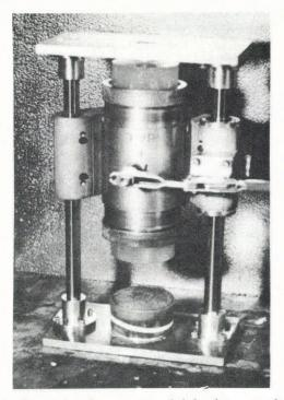
Fig. 1. Carpeted end cap surrounded by latex membrane on the end-capping system described by Cole and others (1985).
