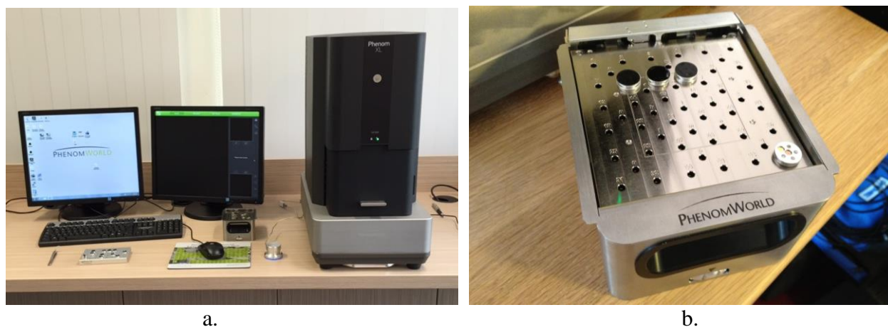
Figure 1. a) Typical benchtop SEM system set-up (Phenom XL with monitor with the microscope control and monitor with four-step GSR interface and EDS/XRM software and b) the multi-sample holder that can handle large specimens.
