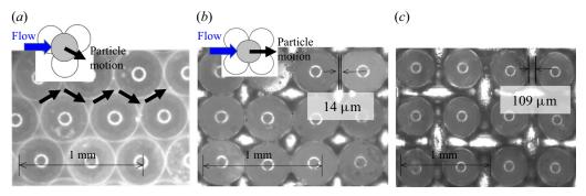
Figure 1. Substrate geometries. Top view on the triangular configuration (*a*), and on the quadratic configuration with spacings (*b*)  $14 \mu m$  and (*c*)  $109 \mu m$ . Main flow direction is from left to right as indicated by the large blue arrows in the sketches. On the triangular arrangement, the bead travels in a zigzag manner along the grooves as indicated by the thick black arrows.
