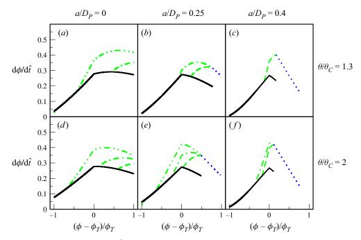
Figure 12. Angular velocity  $d\phi/d\hat{t}$  as a function of the local position  $\phi$  for  $\eta_K = \eta_S$  along the substrate sphere for different spacings  $a/D_P$  and Shields number ratios  $\theta/\theta_C$ . Black solid, green dashed and blue dotted lines indicate rolling, sliding and detached motion, respectively. The different sliding curves refer to friction coefficients  $\eta_K$  of 0.1 (dash-dot-dot), 0.5 (dash-dot) and 1 (simply dashed).
