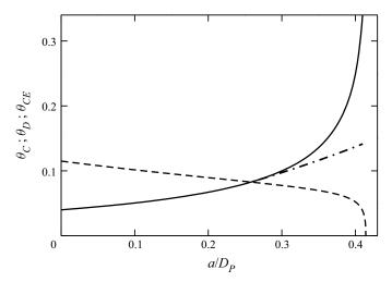
Figure 16. Critical Shields number for detachment  $\theta_D$  (dashed line), for incipient motion from rest  $\theta_C$  (solid line), and for cessation with detachment  $\theta_{CE}$  (dash-dotted line) as functions of substrate spacing  $a/D_P$ . Here,  $\theta_C$  is as according to Agudo *et al.* (2017*a*).
