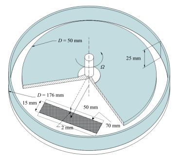
Figure 2. Sketch of the container and the rotating rheometer disk.
