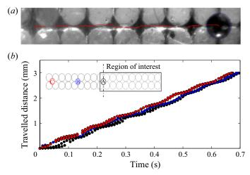
Figure 4. (*a*) Path line of a glass bead during its displacement along seven substrate pockets, and (*b*) particle position as a function of time. Black, red and blue curves represent experiments with the particle placed at the initial positions A, B and C, as indicated in the inset, respectively. The experiments are performed with the less viscous oil at radius 50 mm and at constant Shields number 0.1, corresponding to  $\theta/\theta_C = 2.5$ . Here,  $a/D_P = 0.035$ .
