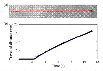
Figure 3. (a) Path line of a glass bead during its displacement along 38 substrate pockets. Flow from left to right. Experiment performed with the less viscous oil. (b) Particle position as a function of time. The dashed line is a linear fit to the data, drawn to guide the eye, and  $a/D_P = 0.035$ ,  $\theta = 0.058$ .
