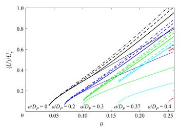
Figure 14. Average bead velocity for different spacings  $a/D_P$  as a function of the Shields number. This solid lines depict purely rolling motion, corresponding to infinite friction coefficients  $\eta_S$ , without flights. Thick solid lines indicate purely rolling motion with flights, while the dash-dot and dashed curves show the additional impact of sliding with friction coefficients  $\eta_S = \eta_K$  of 0.5 and 1, respectively.
