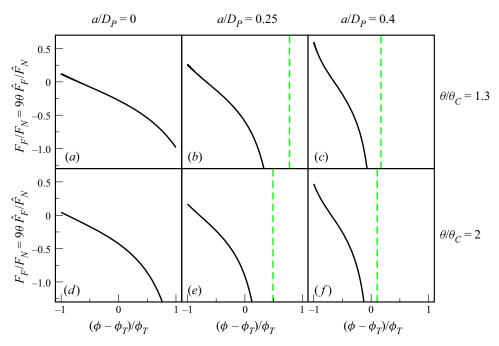
Figure 11. Ratio of tangential force to normal force along the substrate for two Shields number ratios  $\theta/\theta_C$ , and three different substrate spacings. The vertical dashed lines indicate the positions where  $F_N$  becomes zero.
