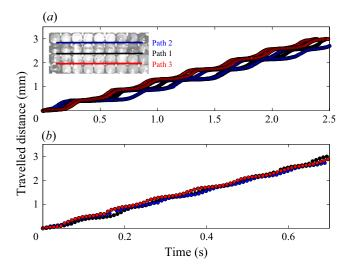
Figure 5. Particle position during its motion along seven substrate pockets on the substrate with narrowest spacing at Shields numbers (a) 0.052 and (b) 0.1, corresponding to  $\theta/\theta_C = 1.3$  and 2.5, respectively. Black, red and blue curves correspond to experimental runs with the bead placed on paths 1, 2 and 3 indicated in the inset, respectively. The experiments are performed using the less viscous oil at radius about 50 mm.
