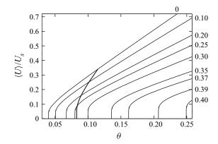
Figure 10. Average velocity of purely rolling beads for different spacings  $a/D_P$  as a function of the Shields number according to (4.20). The respective values for  $a/D_P$  are printed at the ends of the curves. The thick curve indicates the onset of detachment.
