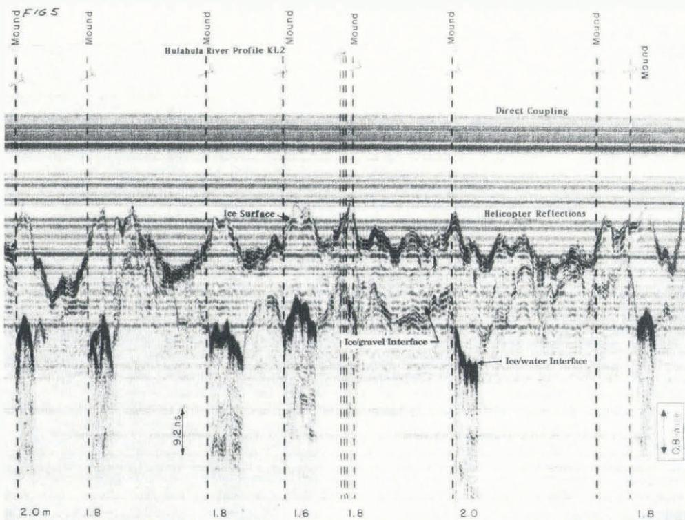
Fig. 3. Short-pulse radar profile taken along the ridges of eight consecutive mounds in Hulahula River. Numbers at the bottom are approximate depths in meters of water under the ridges as interpreted using the ice-depth scale on the graph. "KL2" is one of about 100 such profiles compiled in a CRREL report.
