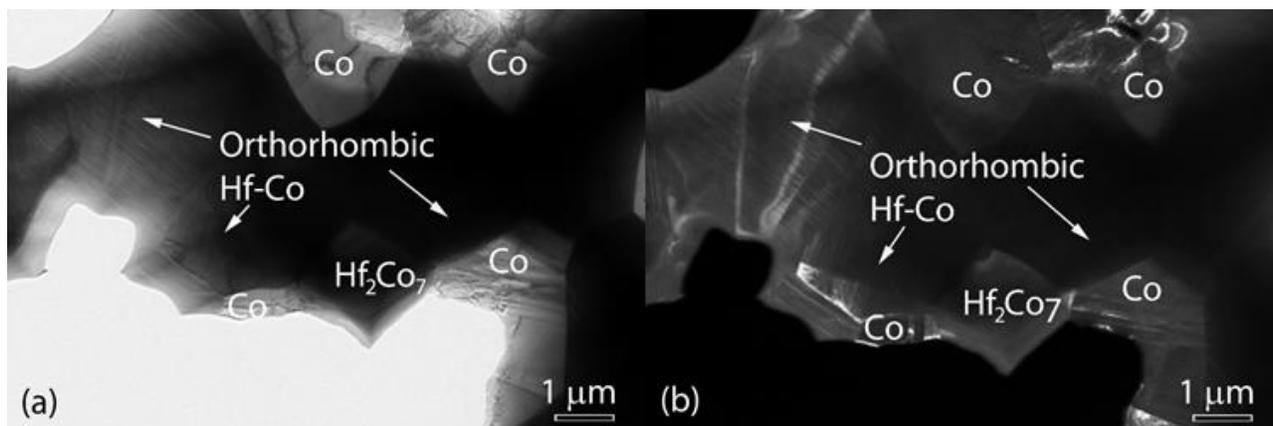
**Figure 1.** (a) BF and (b) DF TEM images of a sample with a nominal composition  $\text{HfCo}_7$ . Grains of the  $\mu$ -phase ( $\text{HfCo}_{6+\delta}$ ), the FCC Co phase, and the  $\text{Hf}_2\text{Co}_7$  phase were marked.
