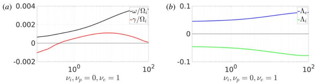
FIGURE 10. The frequency,  $\omega$ , and the growth rate  $\gamma$ , of the ITG instability (a) and associated scaled quasilinear particle fluxes (b) as a function of the ion fraction  $\nu_i$ , in non-neutral electron–antiproton plasma. Parameters as given in the text.
