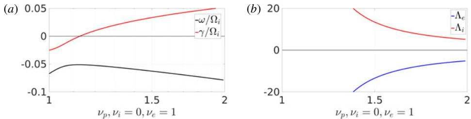
FIGURE 7. The frequency  $\omega$ , and the growth rate  $\gamma$ , of the PTG instability (a) and the associated scaled quasilinear particle fluxes (b) as a function of the positron fraction  $\nu_p$ , in non-neutral pair plasma. We note that in a non-neutral pure pair plasma (i.e. with no ion contamination) it is still possible to have temperature-gradient-driven instabilities as there is no requirement for the electron and positron contributions to cancel. Parameters as given in the text.
