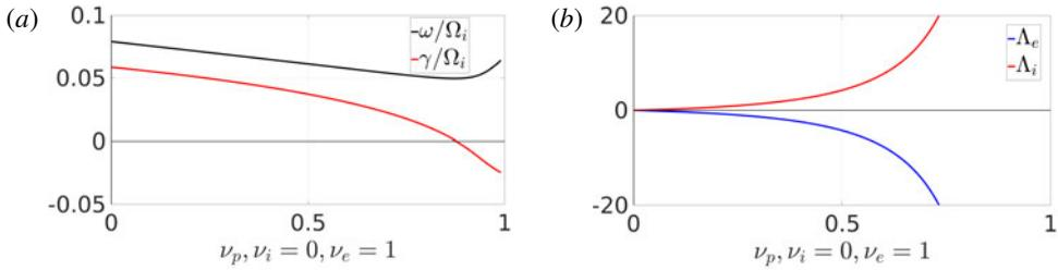
FIGURE 6. The frequency  $\omega$ , and the growth rate  $\gamma$ , of the ETG instability (a) and the associated scaled quasilinear particle fluxes (b) as a function of the positron fraction  $\nu_p$ , in non-neutral pair plasma. We note that in a non-neutral pure pair plasma (i.e. with no ion contamination) it is still possible to have temperature-gradient-driven instabilities as there is no requirement for the electron and positron contributions to cancel. Parameters as given in the text.
