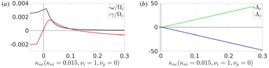
FIGURE 2. The frequency  $\omega$ , and growth rate  $\gamma$ , of the universal mode (a) and the associated scaled quasilinear particle fluxes (b) as a function of the electron density gradient  $\kappa_{ne}$  in a non-neutral electron–ion plasma. The dependence of the growth rate on the density gradient becomes non-monotonic so that a second threshold at large density gradients appears. Parameters as given in the text.
