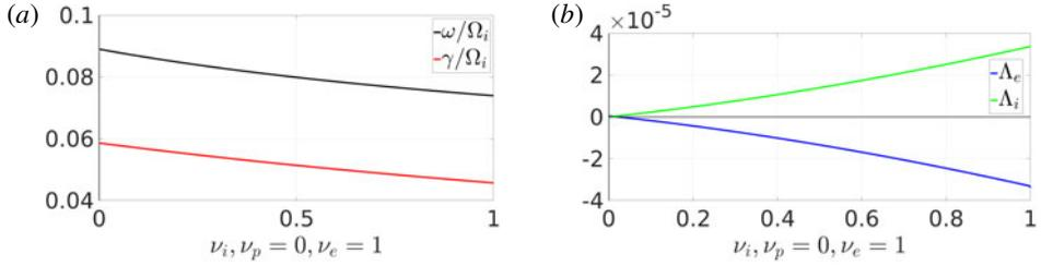
FIGURE 5. The frequency  $\omega$ , and the growth rate  $\gamma$ , of the ETG instability (a) and the associated scaled quasilinear particle fluxes (b) as a function of ion fraction  $\nu_i$ , in a non-neutral electron–ion plasma. Parameters as given in the text.
