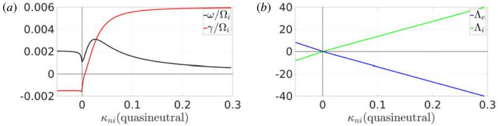
FIGURE 1. The frequency  $\omega$ , and growth rate  $\gamma$ , of the universal mode (a) and the associated scaled quasilinear particle fluxes as defined by (2.24) (b) as a function of the ion density gradient  $\kappa_{ni}$  in a quasineutral electron–ion plasma. One sees that the ion density gradient must be larger than some threshold for the mode to become unstable. The growth rate increases monotonically with the ion density gradient. Parameters as given in the text.
