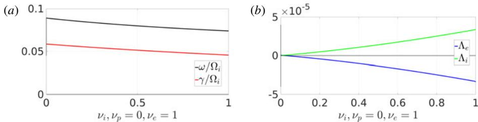
FIGURE 8. The frequency  $\omega$ , and the growth rate  $\gamma$ , of the ETG instability (a) and the associated scaled quasilinear particle fluxes (b) as a function of the antiproton fraction  $\nu_i$ , in non-neutral electron–antiproton plasma. Parameters as given in the text.
