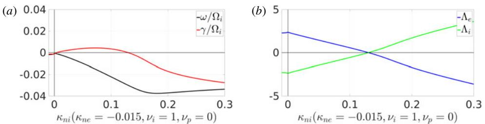
FIGURE 4. The frequency  $\omega$ , and growth rate  $\gamma$ , of the universal mode (a) and the associated scaled quasilinear particle fluxes (b) as a function of the antiproton density gradient  $\kappa_{ni}$  in a non-neutral electron–antiproton plasma. The dependence of the growth rate on the density gradient becomes non-monotonic so that a second threshold at large density gradients appears. Parameters as given in the text.
