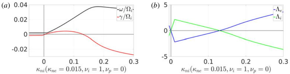
FIGURE 3. The frequency  $\omega$ , and growth rate  $\gamma$ , of the universal mode (a) and the associated scaled quasilinear particle fluxes (b) as a function of the ion density gradient  $\kappa_{ni}$  in a non-neutral electron–ion plasma. The dependence of the growth rate on the density gradient becomes non-monotonic so that a second threshold at large density gradients appears. Parameters as given in the text.
