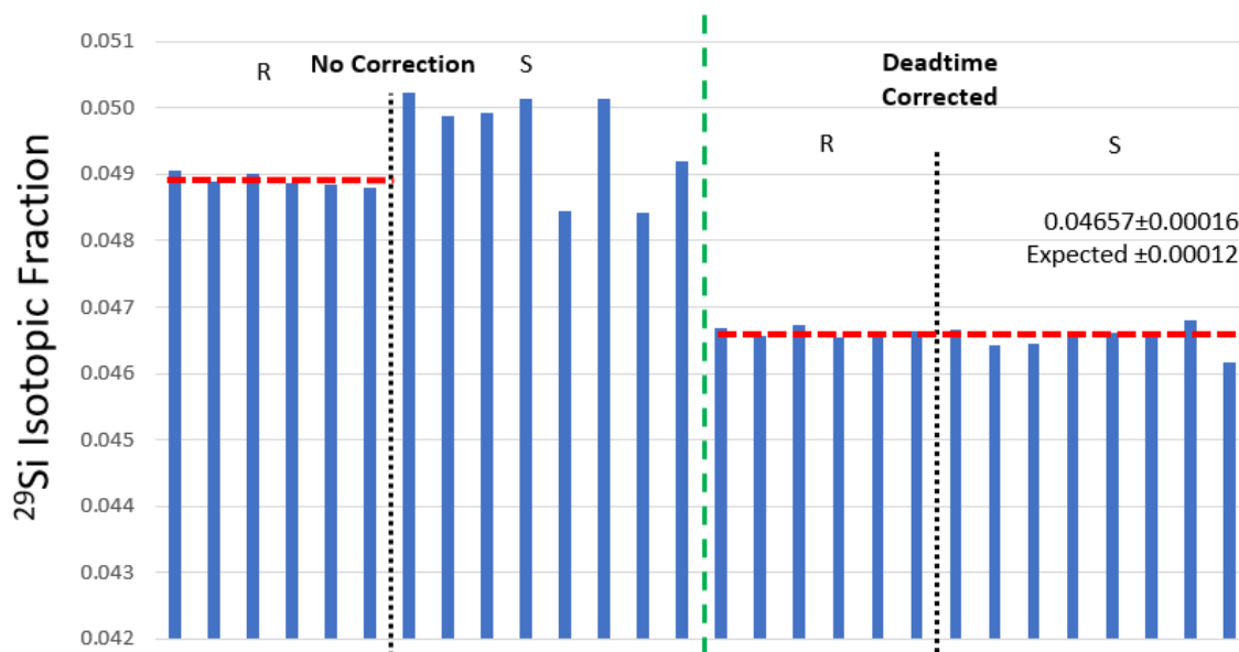
Figure 1. Measurement of the ^{29}\text{Si} isotopic fraction as measured from three LEAP 5000XR and three LEAP 5000XS instruments with some repeats. By utilizing appropriate and consistent data reduction methods, high precision results can be achieved. In this figure the need for appropriate deadtime correction is illustrated. Without deadtime correction (left) the reflectron data is very consistent and has high precision while the straight flight-path data has significant scatter. After deadtime correction, all of the separate measurements agree to nearly the precision predicted by simple propagation of errors and counting statistics ( 0.4567 \pm 0.0016 actual and \pm 0.0012 expected).
