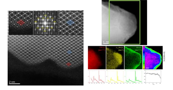
**Figure 1.** HAADF STEM image of LMO viewed along the [110] zone axis. LMO diamonds (blue) are found in the bulk while  $Mn_3O_4$  (red diamond) is visible at the surface. The insets in the image show a higher magnification of the bulk (top right) and surface (top left). An FFT of the full image (top center) is included to indicate the crystal orientation.
