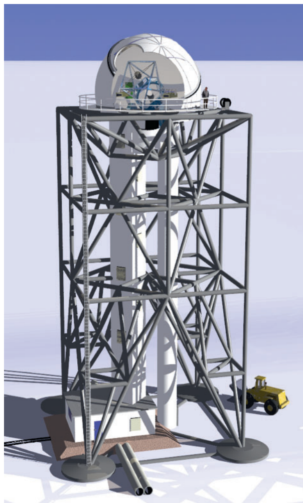
Figure 2 Concept design for the PILOT telescope, enclosure, and tower.
