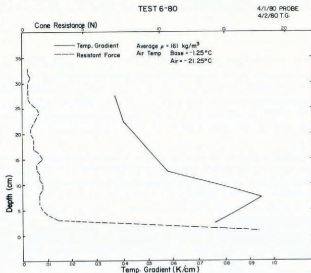
Fig. 1. Correlation between temperature gradient and snow strength within a fairly homogeneous snow-pack. It indicates the tendency for the temperature gradient to decrease with height.
