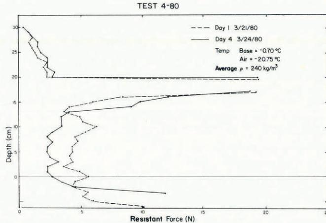
Fig. 7. Change in strength due to a constant temperature gradient for four days. A loss of strength has taken place below the most strongly bonded layer, with little change in strength above.
