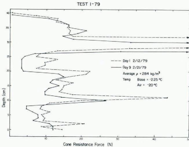
Fig. 6. Changes in strength which developed after nine days of a constant temperature gradient.
