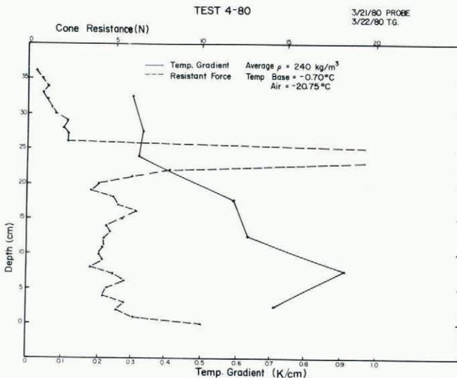
Fig. 3. Correlation between temperature gradient and snow strength in a snow-pack with a distinct resistant layer. The tendency for temperature gradient to decrease with height is demonstrated.
