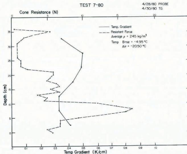
Fig. 4. In inhomogeneous snow, zones of weakness are associated with areas of local maximum temperature gradients and zones of strength with local minimum temperature gradients.
