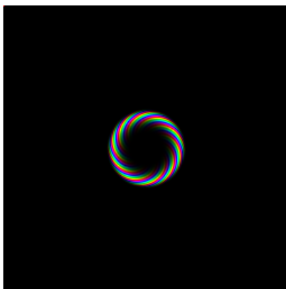
Figure 1: Simulated phase and intensity of +10\hbar vortex subject to the OAM-dependent lens term with b=3 \mu\text{m} , B_0 = 0.01 \text{ T} , R = 10 \mu\text{m} , and beam energy E = 100 \text{ keV} .
