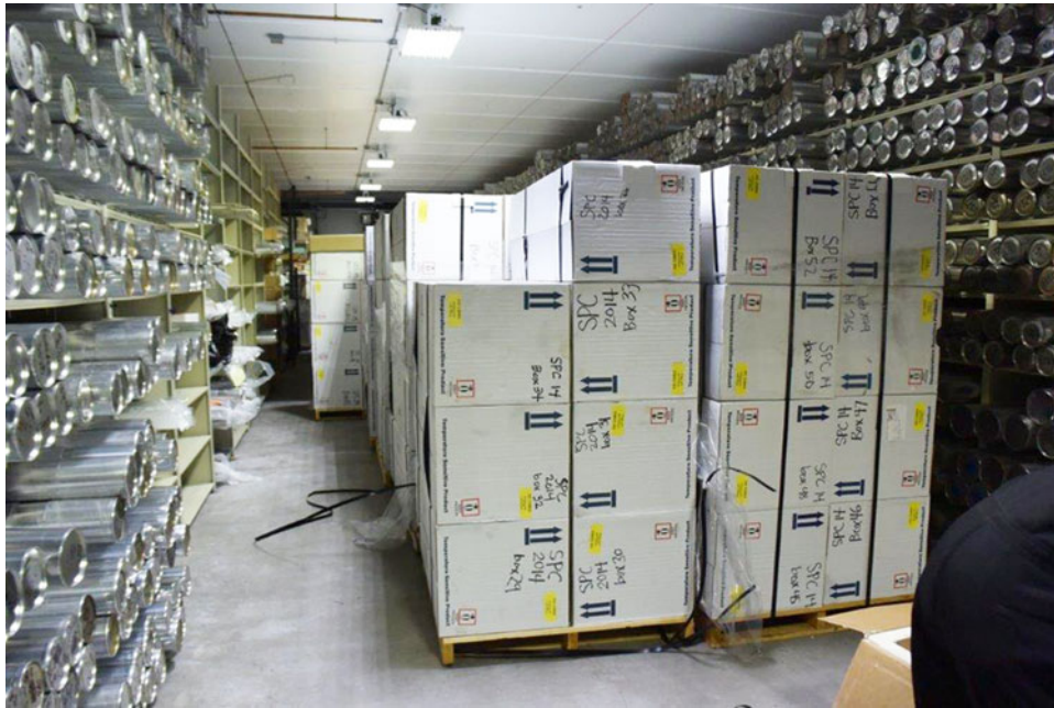
Fig. 11. The retrograded ice cores from the 2014/15 field season sit safely inside the main archive freezer at the NSF-ICF in Denver, Colorado. The temperature inside the main archive freezer is -36^{\circ}\text{C} . Each white box contains five 1 m long sections of the ice core.
