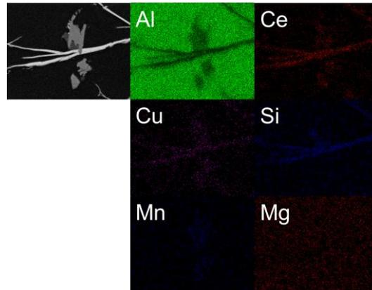
**Figure 4.** EDS-SEM mappings of the as-cast alloy matrix.
