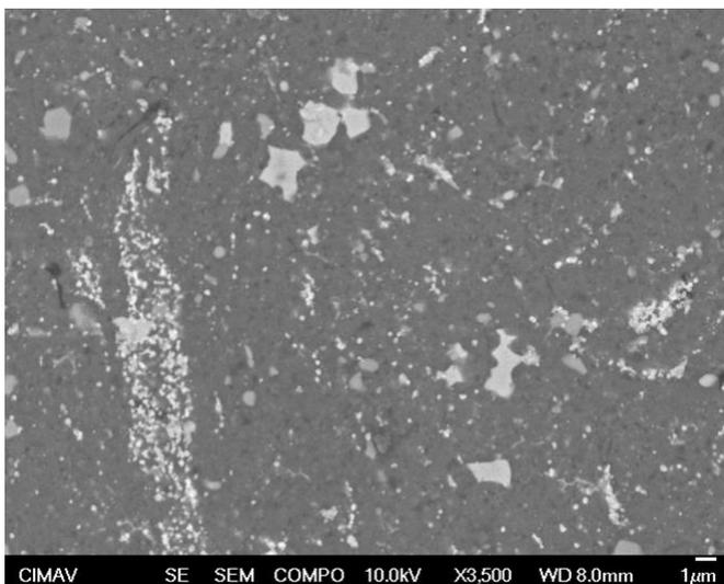
**Figure 5.** SEM image of the sintered A2024+CeO2 alloy.
