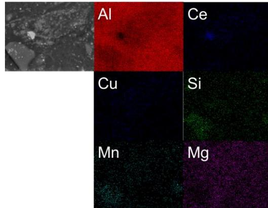
**Figure 6.** EDS-SEM mappings of the sintered alloy matrix.
