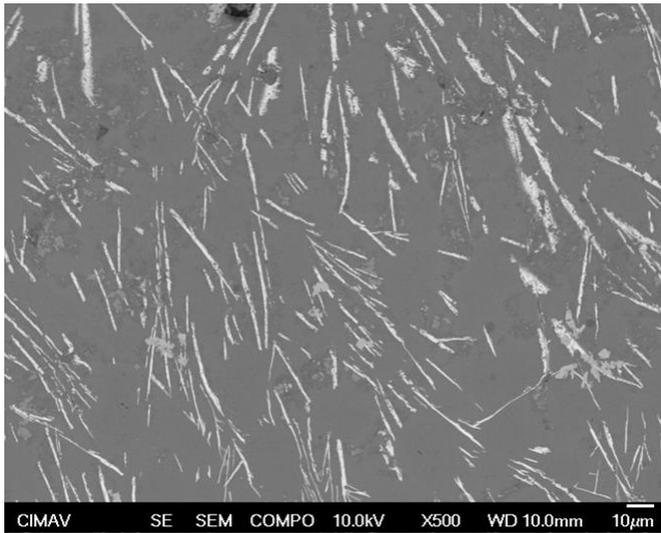
**Figure 3.** SEM image of the A2024+CeO2 as-cast alloy.
