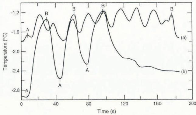
Fig. 5. Basal temperature on right side of plastic ski. (a) Constant-speed ride up Poma lift while cycling the weight on the ski between  $N$  and  $N/2$  with a period of 20 s;  $T_0 = -1.8^\circ\text{C}$ ;  $v_{\text{max}} \approx 2 \text{ m s}^{-1}$ ; hard-packed snow. (b) Three periods of start and stop during a parallel run on a gentle slope;  $T_0 = -2.9^\circ\text{C}$ ;  $v_{\text{max}} \approx 6 \text{ m s}^{-1}$ ; load of  $N$  on hard-packed snow.
