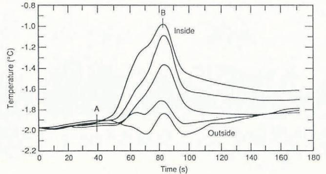
Fig. 8. Basal temperatures from inside to outside of DH skis.  $T_0 = -2^\circ\text{C}$ ;  $v_{\text{max}} \approx 9 \text{ m s}^{-1}$ ; parallel run down gentle slope with load of  $N/2$  on soft, fresh snow.
