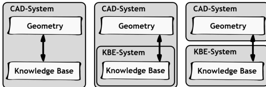
Figure 2. Integration approaches for CAD and KBE - left: integrated; centre: embedded; right: coupled (modified according to VDI, 2017)
