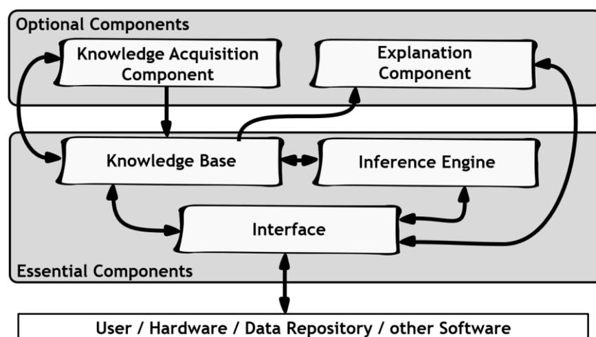
Figure 1. Main components of a knowledge-based system (according to Hopgood, 2012)
