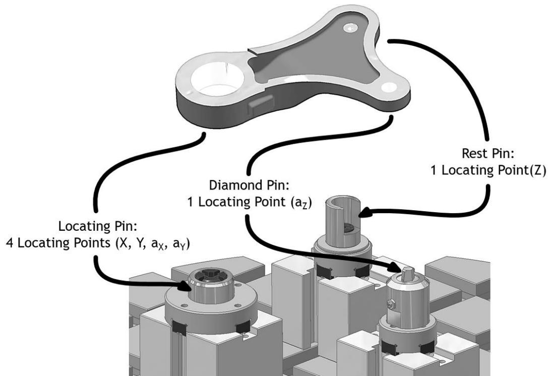
**Figure 6. Main components and locating principle of the modelled jig**
