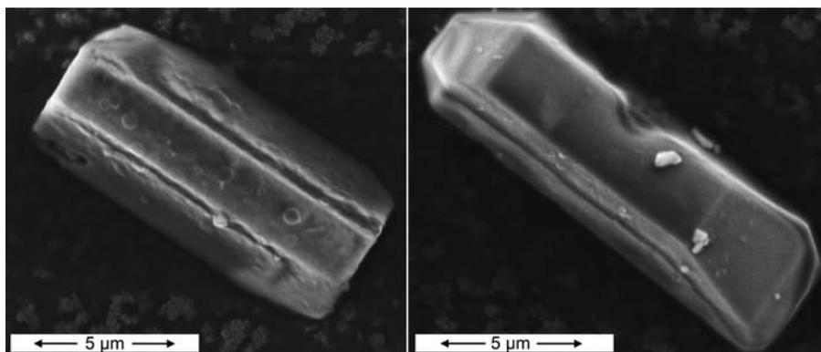
FIG. 2. Scanning electron microscopy – secondary electron images of two larger Pb-lawsonite crystals synthesized from  $\text{PbAl}_2\text{SiO}_{x(7-8)}$  glass and excess water in a piston cylinder experiment at 600°C and 4 GPa.
