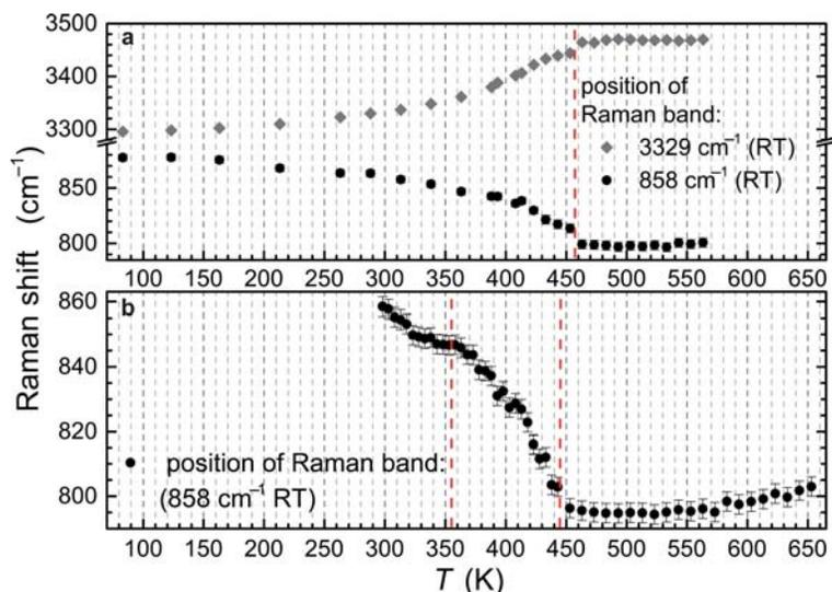
FIG. 5. Band shift analysis of two Raman bands. The band at  $858\text{ cm}^{-1}$  (RT) is assigned to an out-of-plane bending vibration of the hydroxyl group and the band at  $3329\text{ cm}^{-1}$  to a stretching vibration of the OH group. The lower plot shows two, clear, non-uniform changes, one around 355 K and the other around 445 K. The temperature behaviour of (a) and (b) is slightly different, possibly caused by the use of a single crystal (a) and Pb-lawsonite powder (b) for analysis.
