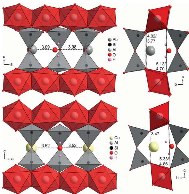
FIG. 12. Comparison of the structural channels of lawsonite (*Pmcn*, 233 K) and Pb-lawsonite (*Pbnm*, 298 K) hosting the Ca/Pb cation and the H<sub>2</sub>O molecule, in two different orientations. Numbers denote the interatomic distances in Å. Note the straightened Si–O–Si angle in Pb-lawsonite, resulting in a more circular cross-section of the channel.
