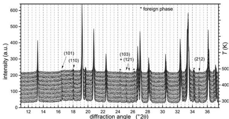
FIG. 7. Powder XRD patterns of Pb-lawsonite ( $T = 298$  to  $498$  K) showing the phase transition from space group *Pbnm* to *Cmcm* around 450 K. The XRD patterns were smoothed and vertically offset to enhance the visibility of the small diffraction peaks. Arrows indicate a number of weak, critical reflections and their indices.
