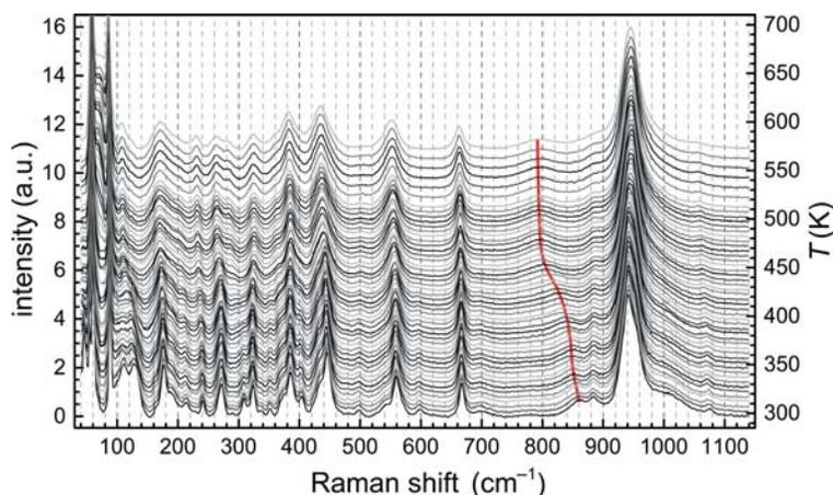
FIG. 4. Temperature-dependent Raman spectra of Pb-lawsonite from 298 to 573 K showing the vibrations of the  $\text{Si}_2\text{O}_7$  groups and  $\text{AlO}_6$  octahedra as well as lattice vibrations. Spectra are vertically offset. The bold line at  $\approx 790\text{--}860\text{ cm}^{-1}$  indicates the maximum of the  $\gamma\text{-OH}$  vibrational band.
