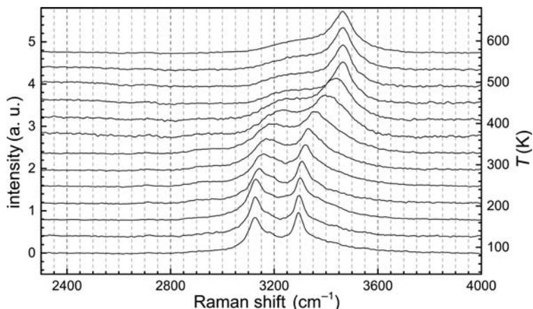
FIG. 3. Temperature-dependent Raman spectra of Pb-lawsonite from 83 to 573 K showing stretching vibrations of the hydroxyl groups and the  $\text{H}_2\text{O}$  molecule. Spectra are vertically offset and smoothed only for presentation.
