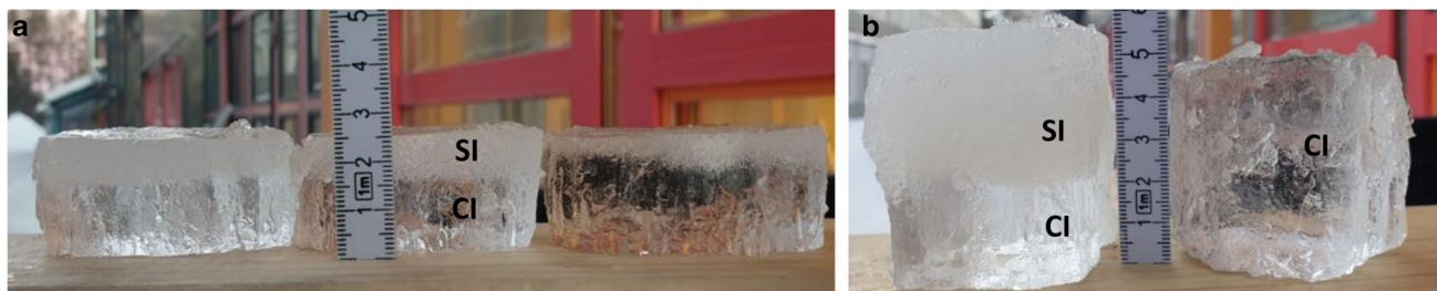
Figure 3. Examples of ice samples. (a) Three ice samples consisting of both congelation and snow ice; (b) the first sample consists of SI and CI underneath, while the second sample only of CI.
