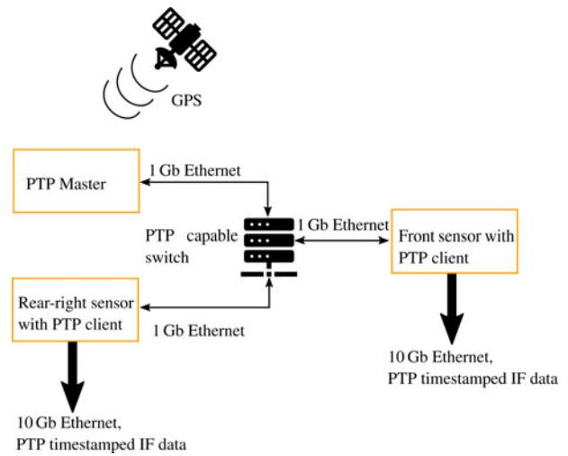
**Fig. 6.** PTP network architecture for accurate time synchronization between the front (calculate trajectory) and rear-right (SAR measurements) radar sensor.
