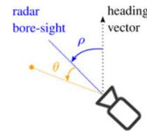
**Fig. 4.** Generalized radar mounting position along with a visual definition of the heading vector, the angle between the heading vector and the radar bore-sight ( $\rho$ ) and the angle between the radar bore-sight and the target ( $\theta$ ).
