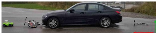
**Fig. 12.** The first measurement scenario. Red arrow indicates the driving direction and the green arrow shows the direction of the SAR sensor bore-sight.
