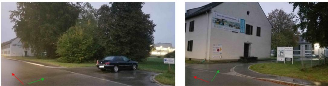
**Fig. 17.** Measurement scenario with various target objects and a trajectory of 100 m. The two pictures show different portions of the same measurement trajectory. (a) Initial part of the measurement involving a parked car, curved kerb, and some trees. (b) Latter part of the measurement consisting of a perpendicular fence, a sign board, and a building.
