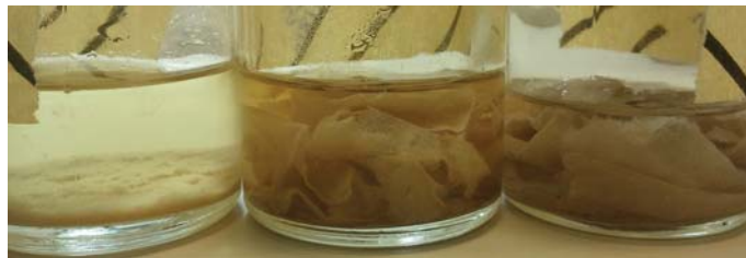
FIG. 3. The triplicate of the tissue microcosms, incubated for 30 months at 25°C and in the presence of Ca(OH) 2 at saturation. Samples 1, 2 and 3 are shown from left to right.
