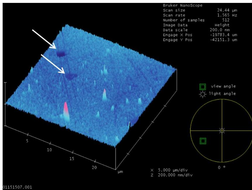
**Figure 1.** Atomic force microscope image of two pinholes in the surface of glass sample coated with ~25nm of TiO<sub>2</sub> ALD.
