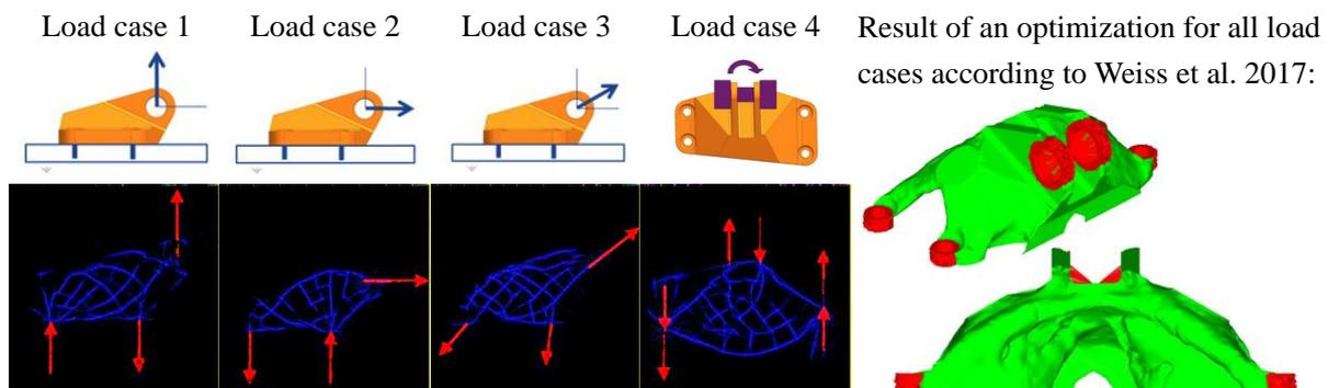
Figure 8: Comparison of the results of an optimization with the new method and a computer-aided optimization according to (Weiss et al., 2017)
