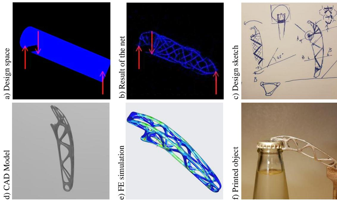
Figure 9: Design process for a bottle opener using the new design tool
