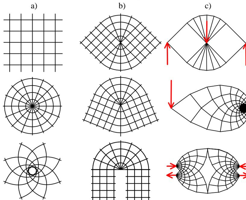
Figure 2: a) Basic forms of the main strain fields according to (Wiedemann, 2007); b) Deformation-compatible combinations according to (Wiedemann, 2007); c) Michell structures for various load cases according to (Michell, 1904)
