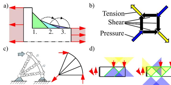
Figure 3: a) Tension triangles (modified from Sauer, 2008); b) Shear square (modified from Mattheck, 2010); c) Comparison of a rope construction (modified from Mattheck, 2010) with a Michell structure; d) The use of force cones to deduce a topology (modified from Posner *et al.*, 2014)
