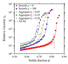
Figure 2. Divergence of the relative viscosity  $\eta_r$  with area fraction  $\phi$  at  $\dot{\gamma}^* = \infty$  for each of the suspension types explored. Shown in dashed lines are fits to  $\eta_r = v(1 - \phi/\phi_m)^{-\lambda}$ . The maximum solid fractions for smooth particles  $\mu = (0, 100)$  and aggregates with  $k_r = (0.05, 0.10, 0.20)$  are, respectively,  $\phi_m = (0.84, 0.77, 0.74, 0.71, 0.69)$  (see table 1).
