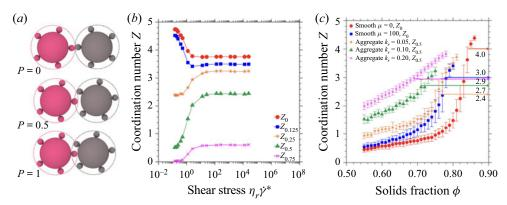
Figure 5. Mechanical coordination number Z for smooth and aggregate particle suspensions. (a) Sketches of the relative particle positions for various values of the interdigitation fraction P; (b) The coordination number measured by different criteria of interlocking, for particles with  $k_r = 0.20$ ,  $\phi = 0.62$  and  $\rho = 3k_ra_h$ ; (c) The coordination number  $(Z, Z_{0.5})$  measured at different  $\phi$  for smooth and aggregate particles (isostatic points depicted by arrows).
