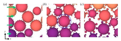
Figure 1. Schematic of aggregate particles (coloured by particle). Shown are suspensions with asperity sizes  $k_r = (a) \ 0.05$ ;  $(b) \ 0.10$ ;  $(c) \ 0.20$ . Green arrows indicate the imposed velocity profile  $u_x(y) = \dot{\gamma} y$ . Blue dashed circle represents contact with P = 0 (see (3.1)).
