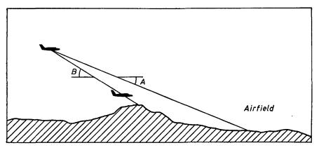
FIG. 1. The gradient of descent and gradient of sight-line
