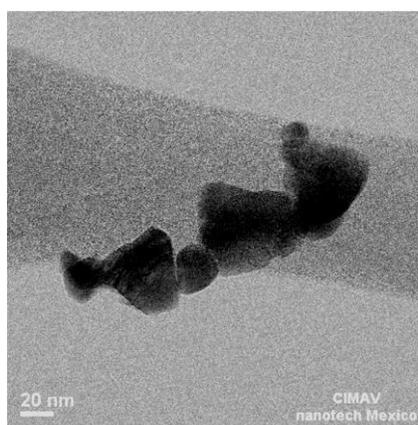
**Fig. 3** HRTEM micrograph of Fe doped ZnO Nanofiber
