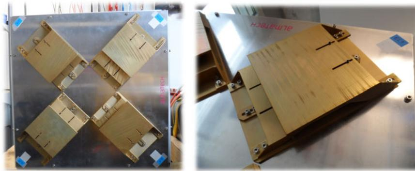
Fig. 10. Simplified radiating elements manufactured and fastened to the cube representing the satellite body.
