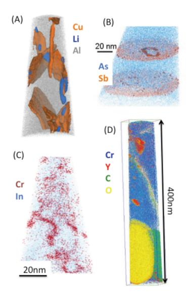
FIG. 1. 3D reconstructions of (A) Cu-rich aand Li-rich precipitates in an Al alloy, (B) quantum rings in GaAs/GaSb structures. (C) Cr distribution in Cr-doped indium oxide and (D) Cr-depleted grain boundaries and second phases in an oxide dispersion strengthened steel.
