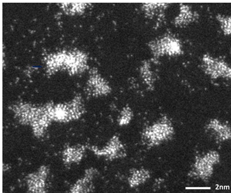
Fig.1: Single atom and raft imaging of Pt under reaction conditions (Pt/C/H<sub>2</sub>); atoms imaged at 0.11±0.01nm diam in HAADF ESTEM
