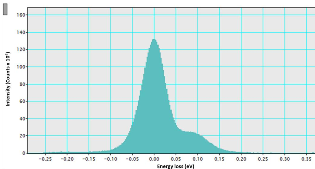
**Figure 1.** EELS spectrum of *h*-BN collected on the Themis Z at 60kV. The spectrum is summed from several pixels of a spectrum image. The convergence and collection angles were 27.4 and 22.8 mrad, with a spectrometer entrance aperture of 2.5mm and a dispersion of 0.002eV per channel. The FWHM is 69meV.
