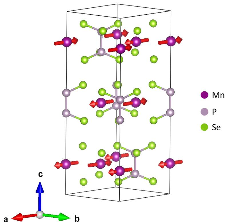
**Figure 2.** The structure of MnPSe<sub>3</sub>. The red arrows in the manganese atoms indicate the direction of magnetic spin. MnPSe<sub>3</sub> is antiferromagnetically ordered below 74 K.
