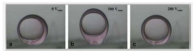
Figure 3. Sequence of video frames showing accelerated centering of inner silicone oil droplet by intentionally inducing elongation of the outer shell. (a) Before application of voltage; (b) a strong electric field E_0 = 23 \text{ kV}/\text{m} at 100 kHz is applied for \sim 15 \text{ s} ; (c) field strength is reduced to 13 \text{kV}/\text{m} . The time required for the inner droplet to achieve centering is reduced from \sim 80 to \sim 45 \text{ s} and this lower field strength sustains the concentric condition indefinitely (taken from Ref. [72]).
