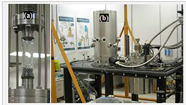
Figure 6. Fluidized bed with a massive of Au/Pd-coated PAMS shells of a 4 mm diameter. (a) Bed is out of the cryostat; (b) bed is inside the cryostat. Bed fluidized at 9 K (taken from Ref. [54]).
