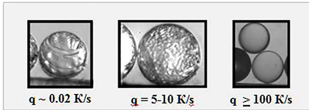
Figure 21. Different cooling rates give rise to the cryogenic H 2 -layer formation with a different granularity. No additives are used in these experiments.
