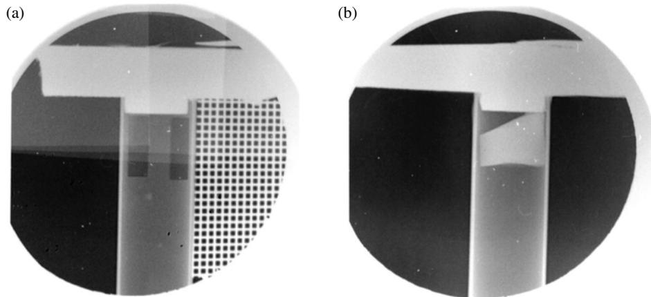
**Figure 10.** Sample backlighter images showing: (a) the PI tube with the quartz/steel obstacle at the top, the diagnostic slits cut in to the tube and the gold resolution grid attached to the target and (b) the PI tube with the quartz/steel obstacle at the top and a low-density foam insert below the stop.
