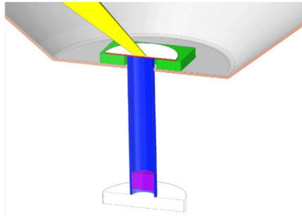
**Figure 3.** Shows a 3D CAD cut away of the target and indicates the positions of the pusher foil position and also shows the foam insert at the bottom of the tube.
