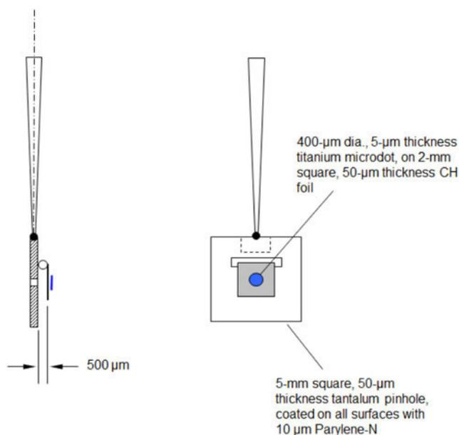
**Figure 8.** The backlighter target design.
