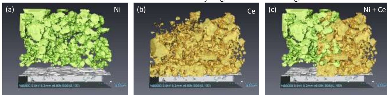
Figure 2. 3D reconstruction of (a) Ni (b) Ce and (c) Ni+Ce. BSE image contrast was used to identify the phase differences. For 3D analysis, 40 kV FIB with Ga-ions along with BSE imaging were used on newly created surfaces at a separation of 100nm.
