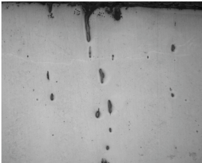
Figure 2. As polished micrograph (100x original magnification) of shaft just below the fracture plane.
