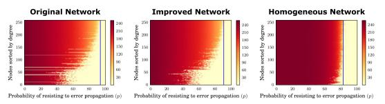
**Figure 6.** Simulations of cascades on the three networks. The blue line represents the threshold probability needed for which no node can activate a catastrophic cascade. The threshold for the original network is around 94%, for the improved network is around 91%, and for the homogeneous network is around 83%.
