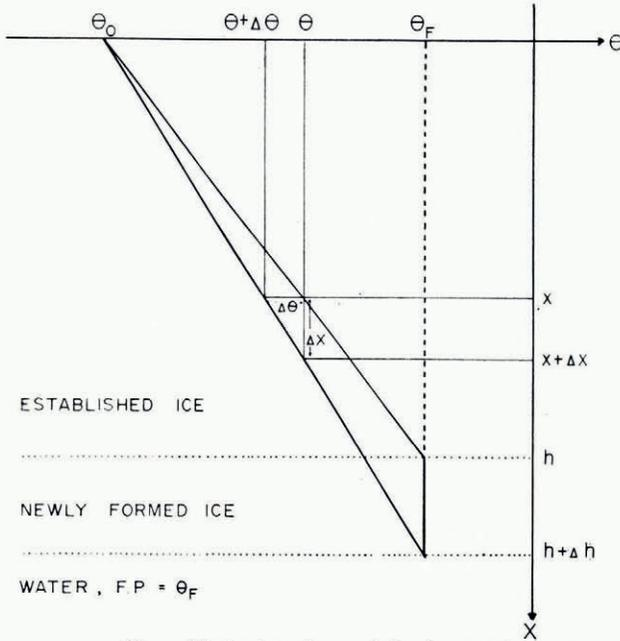
Fig. 1. Temperature changes during ice growth
