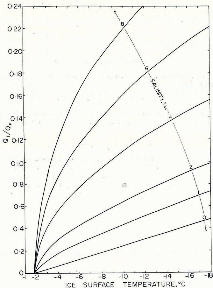
Fig. 2. Corrections to Stefan's simple ice-growth equation. Ratio of contributions to surface heat flux from ice-cover cooling  $Q_i$  to that for new ice forming  $Q_F$  as a function of ice surface temperature for various salinities
