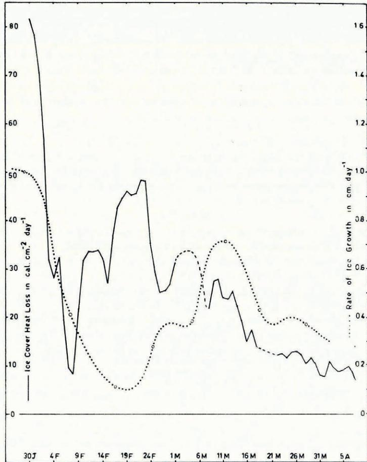
Fig. 3. Ice surface heat flux and growth rate of sea ice in Hudson Bay near Churchill, Manitoba, January to April 1961
