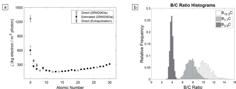
**Figure 1.** (a) Experimentally determined  $\zeta$ -factors and (b) determined boron carbide stoichiometries of three bulk samples.
