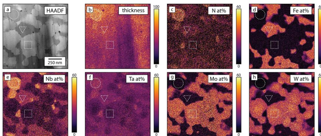
**Figure 2.** STEM-XEDS spectral image of a mechanically alloyed NbMoTaW CCA after annealing at 1200 °C for 1000 hours: (a) HAADF micrograph, (b) thickness (nm), (c) N at.%, (d) Fe at.%, (e) Nb at.%, (f) Mo at.%, (g) Ta at.%, and (h) W at.%. The microstructure contained a W(Mo) BCC solid solution (square), Fe-Ta-Nb-rich M<sub>6</sub>N η-nitride (triangle), and a Nb-Ta-rich M<sub>2</sub>N heminitride (circle). Mo and W were correlated just as Ta and Nb were correlated.
