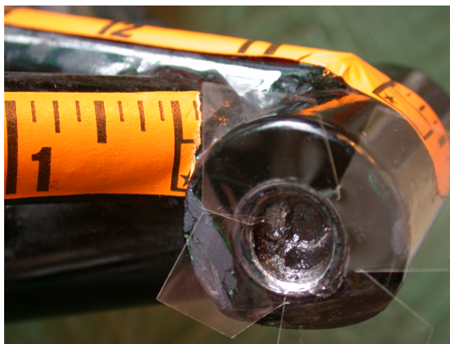
Figure 4. Replication of the bolt fractured surface.
