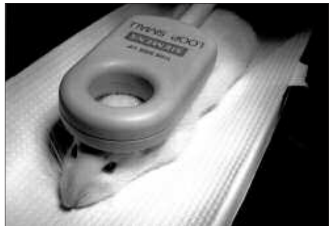
Figure 1: Illustration of the setup used for imaging. An anesthetised Fischer rat rests prone inside the magnet with the small loop antenna simply laid on its head.
