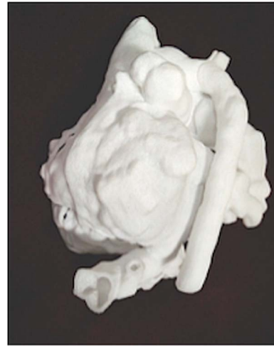
Figure 3. SLS Nylon heart model.
