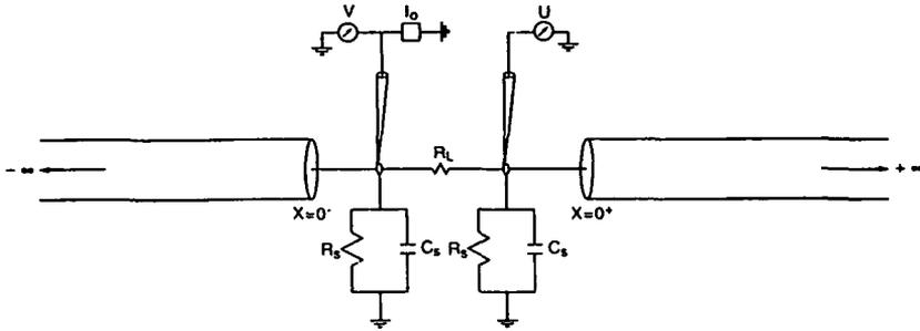
FIGURE 2. Electrophysiological experiment consisting of a pulse of current injected into the soma of a single neuron and a measure of the voltage response (at early times) in the coupled neuron, recorded in a system of two electronically coupled neurons. An emphasis on the somatic coupling between each neuron is given, since the dendritic terminals are assumed to be at an infinite electronic distance from the soma.
