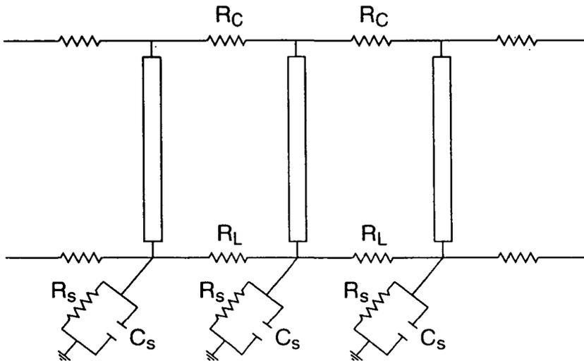
FIGURE 1. A network of electronically coupled neurons each represented by an equivalent cylinder for the dendritic tree (and axon), and a RC-circuit for the cell body (soma). Each neuron is coupled to another neuron at the soma by a resistance ( $R_L$ ) and in the dendrites by a resistance ( $R_C$ ).
