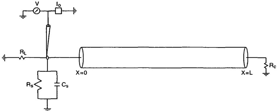
FIGURE 3. Electrophysiological experiment consisting of a pulse of current injected into the soma of a single neuron and a measure of the voltage response recorded. The effects of current leakage due to somatic and dendritic gap-junctions have been approximated with resistances  $R_L$  and  $R_c$  respectively.
