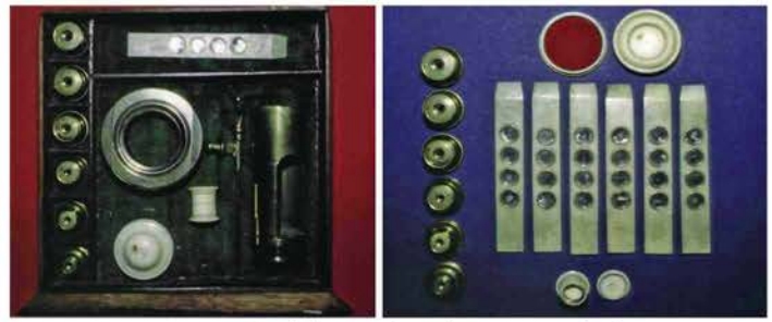
Figure 3. Baize-lined draw with 6 objectives, circular brass spring tige, stage forceps, ivory sliders, ivory box with talcs and split brass rings, lieberkuhn holder and circular ivory box with lieberkuhn.
