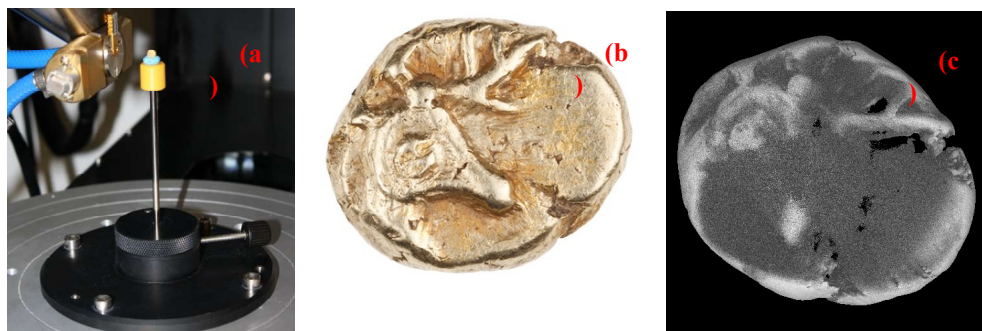
Figure 1. (a) Photograph of a Phanes electrum coin mounted for \mu CT analysis; (b) Photograph of the obverse side of the Phanes electrum coin with a stag head to right; (c) \mu CT image of the surface of the coin in (b) showing the surface profile as well as cracks near the antler at the coin edge.
