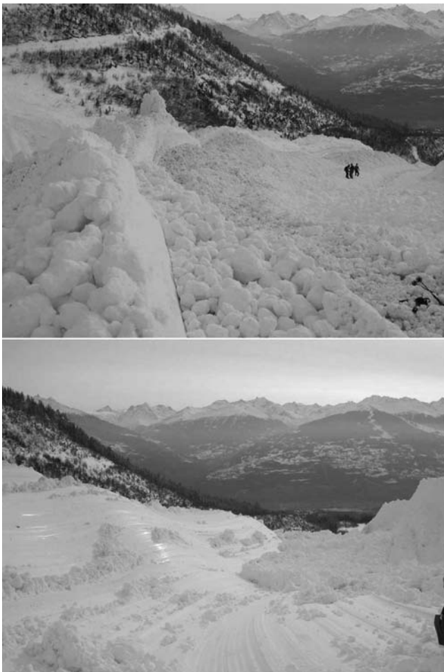
Fig. 1. Top: The granular deposits of a large snow avalanche released at the Swiss Vallée de la Sionne test site. The snow granules are 10–20 cm in size. Bottom: The basal sliding surface of a large snow avalanche. Note the shining ice layer produced by basal friction. The ice layer is several millimetres thick. A shovel is located at the right of the bottom picture. Such observations indicate that basal sliding, viscous shearing and inelastic collisions are the primary energy-dissipation processes.
