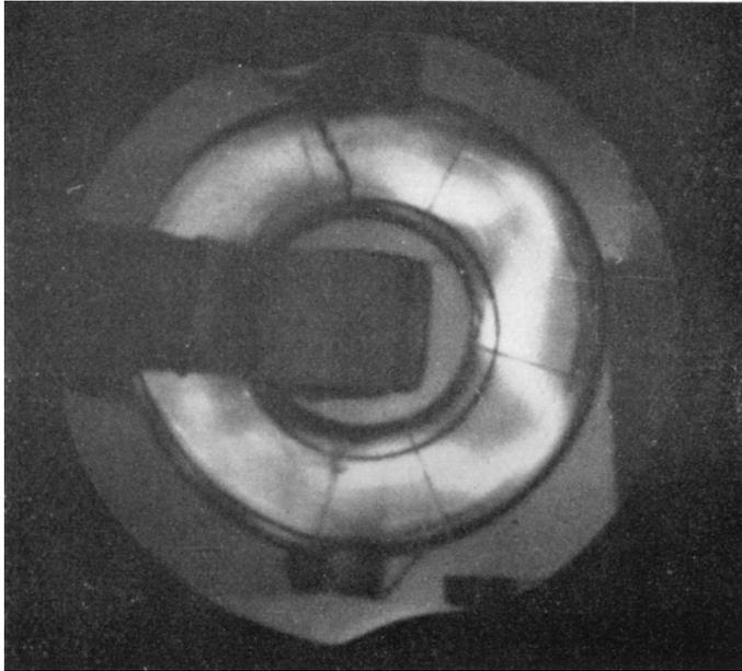
Plate II. Gaseous discharge in a toroidal tube without electrodes. The gas forms the secondary of a pulse transformer. For strong currents a helical configuration arises as seen from the picture.
